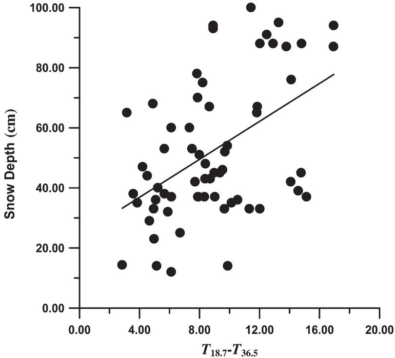
Figure 2. The regression curve used to derive the relation between brightness temperature and snow depth over the north-western Himalayas. The  $T_b$  difference for the 18.7 GHz and 36.5 GHz channels of AMSR-E is plotted on the  $x$ -axis.
